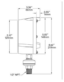
Other ranges and connection sizes (3/4" NPTM, 1" NPTM, 1/2" NPTF) available upon request. Other fills available. Pin stop at 6 o'clock position available. For options, attach suffix to end of order code: i.e. PTR5070-SF45 for SILICONE-FILLED GAUGE CASE.
